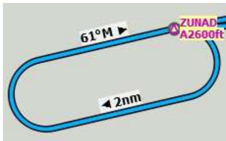
A hold with 2 NM straight segment length. Enter and exit at ZUNAD and fly at or above 2,600 ft. Course is 61° magnetic degrees.
