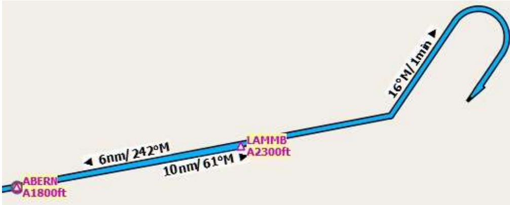
A procedure turn. Fly at least one minute outbound 61° from ABERN, turn left to 16°, fly one minute, turn 180° and fly to LAMMB, then 242° to ABERN.
