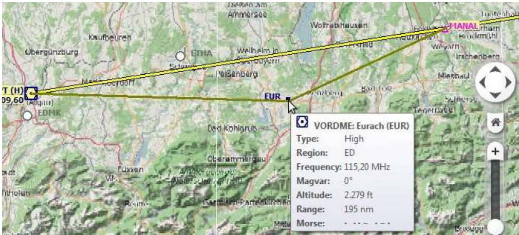
Inserting a navaid into a flight plan leg by clicking and moving the leg line. A tool tip for the navaid is shown.
