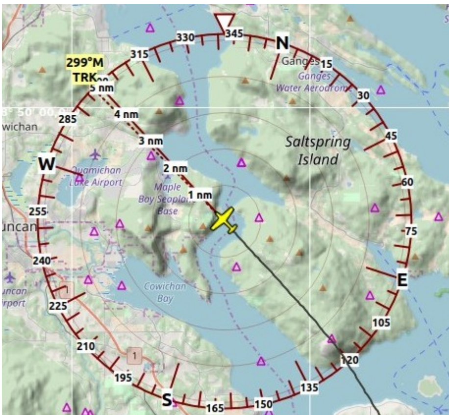
Compass rose centered around user aircraft. No flight plan loaded. Therefore, heading and next waypoint indicators hidden.
